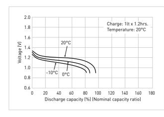
Self-discharge is affected by the temperature at which the batteries are left standing and the length of time during which they are left standing. It increases in proportion as the temperature or the shelf-standing time increases. Panasonic's Ni-MH batteries have excellent self-discharge characteristics.
