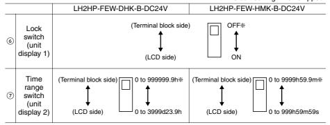
Notes: 1. Make the switch setting before installing to panel.
