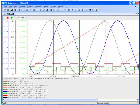
The FP Data Analyzer can be connected to any Panasonic PLC by utilizing the integrated MEWNET Manager, for instance via any COM-port. Recording and analyzing remote PLCs, sensors, actuators, etc. via LAN or modem is just a matter of seconds. Open the MEWNET Manager Communication Setup Dialog, select Ethernet or Modem and enter your parameters.
