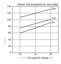
1-(2). Coil temperature rise (at 85°C 185°F) Sample: ACT212, 3pcs. Contact carrying current: 0A, 10A, 20A
