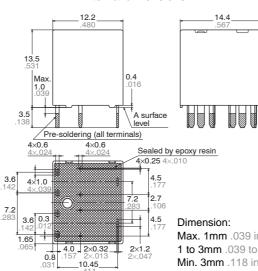
Tolerance Max. 1mm .039 inch: ±0.1 ±.004 1 to 3mm .039 to .118 inch:  $\pm 0.2 \pm .008$ Min. 3mm .118 inch: ±0.3 ±.012
