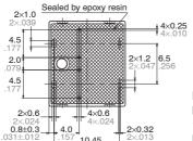
Dimension: Tolerance Max. 1mm .039 inch:  $\pm 0.1 \pm .004$ 1 to 3mm .039 to .118 inch: ±0.2 ±.008 Min. 3mm .118 inch: ±0.3 ±.012
