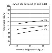
1.-(4) Coil temperature rise (at 85°C 185°F) Sample: ACJ2212, 3pcs Measured portion: Inside the coil Contact carrying current: 10A, 15A, 20A Ambient temperature: 85°C 185°F
