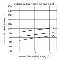
1.-(3) Coil temperature rise (at room temperature)
