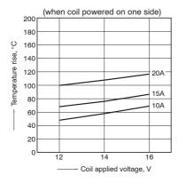
1.-(5) Coil temperature rise (at room temperature)
