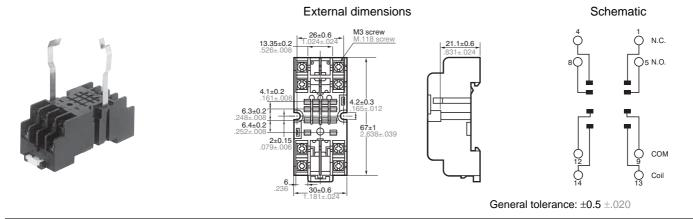
HC3-high DIN rail terminal socket (HC3-SFD-K)
