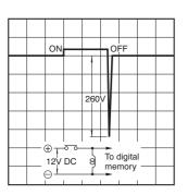
1.-(2) DC coil surge voltage waveform (with diode) Diode characteristics; Reverse breakdown voltage: 1,000V, Forward current: 1A
