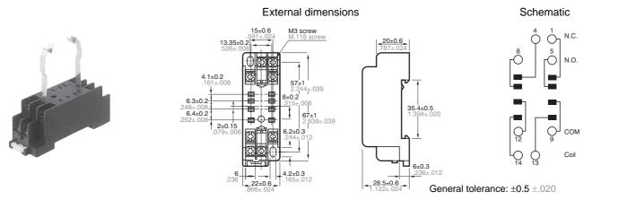
A HC2-high DIN rail terminal socket (HC2-SFD-K)
