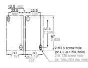
Panel hole dimensions for side-by-side mounting
