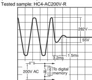
1.-(2) AC coil surge voltage waveform (without CR circuit)
