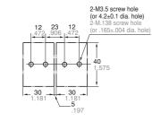
Panel hole dimensions for side-by-side mounting
