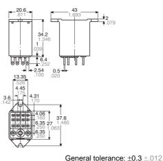
The diagrams show the external dimensions of the 4 Form C and 4-pole bifurcated (twin) types. For 1 Form C, 2 Form C, and 3 Form C, see diagrams at plug-in types (only the terminals are different).
