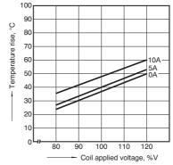
3.-(8) Coil temperature rise (4 Form C, DC type) Measured portion: Inside the coil Ambient temperature: 17 to 18°C 62 to 64°F
