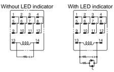
Diagrams show the external dimensions and schematic of the 4 Form C and 4-pole bifurcated (twin) types. For the 1 Form C, 2 Form C, and 3 Form C types, only the terminals differ. The dimensions of the terminal are the same as for standard type HC relays.
