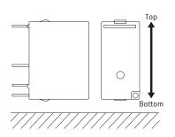
When installing with the relay terminals parallel to the ground, the contact terminals at the bottom and the coil terminals at the top, component friction will occur after numerous switching actions or due to vibration in the non-excitation state. Since this may cause the relay to stop functioning when the pick-up voltage increases even if the nominal voltage is applied, please do not install using this orientation.
