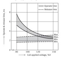
3.-(2) Operate & release time (1 Form C type) Tested sample : JQ1-24V-F, 25 pcs.
