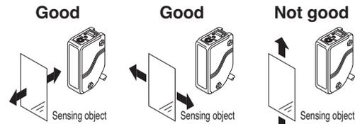
Do not make the sensor detect an object in this direction because it may cause unstable operation.
