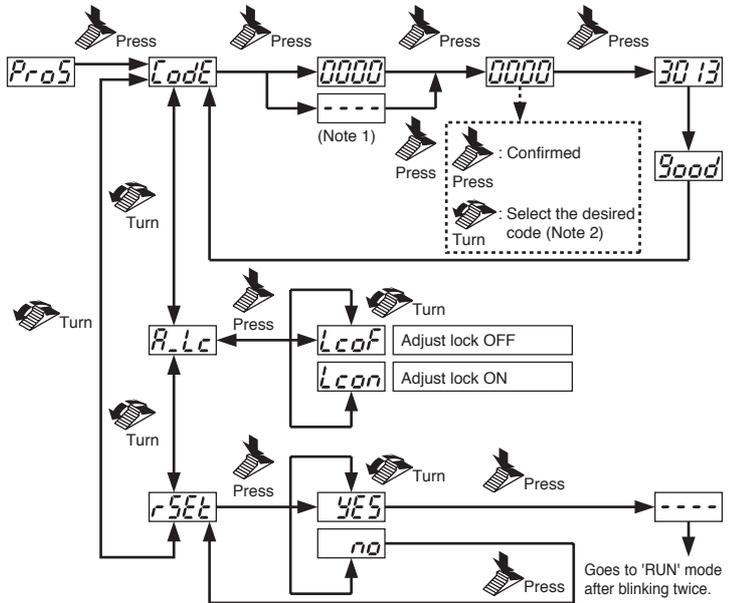
Notes: 1) When any code other than the codes given in the Code setting table below is used, ' - ' is displayed. The factory setting is '0004'.
