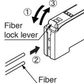
Notes: 1) In case the fiber cables are not inserted to a position where they stop, the sensing range reduces. In case of a flexible fiber, take care that it may bend inside the amplifier, during insertion.
