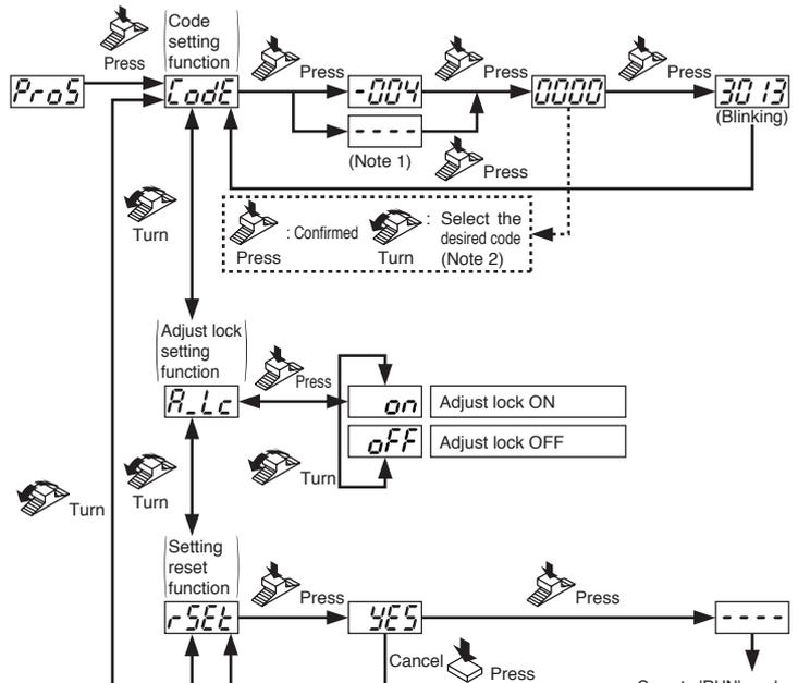
Notes: 1) When any code other than the codes given in the code setting table below is used, '-' is displayed.
