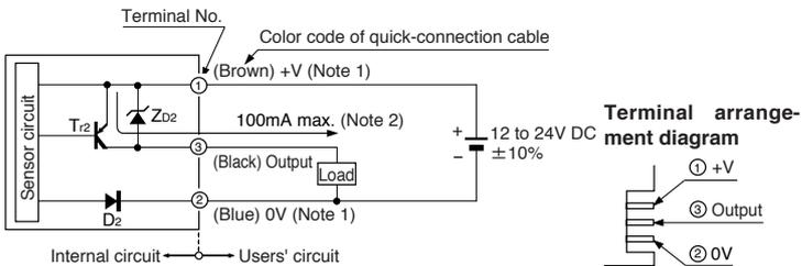
Notes: 1) The quick-connection sub cable does not have +V (brown) and 0V (blue). The power is supplied from the connector of the main cable.
