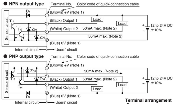
Notes: 1) The quick-connection sub cable does not have +V (brown) and 0V (blue). The power is supplied from the connector of the main cable.
