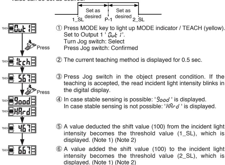
Notes: 1) The shift value 100 digits is the initial value. The shift value can be changed in PRO mode. Furthermore, 'digit' or 'percent' can be selected. For the setting method refer to '13 PRO MODE · PRO6 mode setting'.
