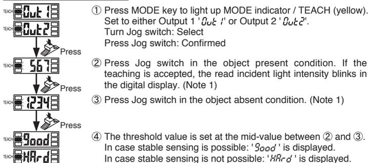
Note: In case of using the fibers, if Jog switch is pressed in the object absent condition at ② and ③, the sensitivity is set to the maximum.
