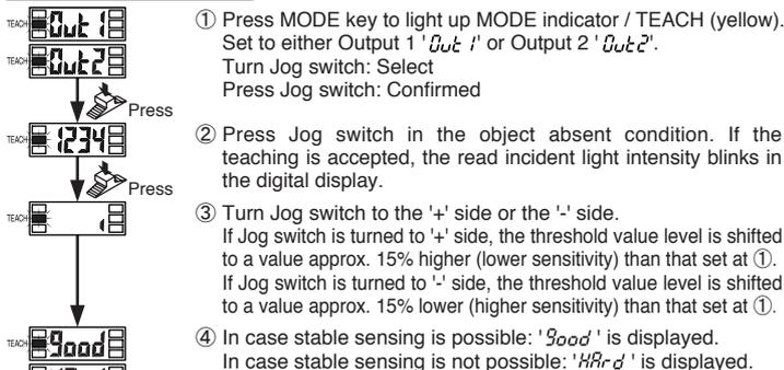
Note: The approx. 15% amount of shift is the initial value. The amount of shift can be changed in the PRO mode from approx. 0 to 80% (5% step). For the setting method refer to '13 PRO MODE · PRO1 mode setting'.
