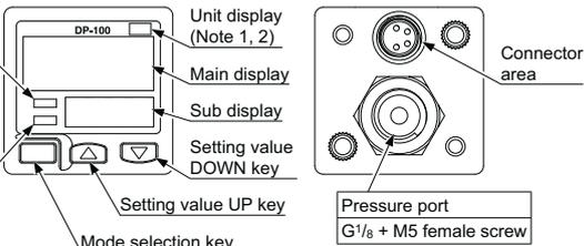
Note: If set the pressure unit other than 'MPa' or 'kPa', attach the unit switching label corresponds to the set pressure unit.
