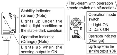
Note: Not incorporated on the thru-beam type sensor emitter.
