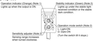
Notes: 1) It is the power indicator (orange) (lights up when the power is ON) for the emitter.
