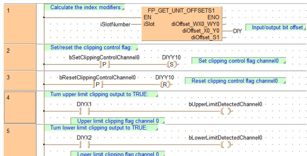
When bSetClippingControlChannel0 turns to TRUE, the limit alarm function on channel 0 is activated. When bResetClippingControlChannel0 turns to TRUE, the function is deactivated.
