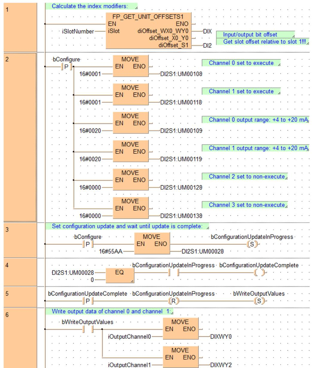
When `bConfigure` turns to TRUE and `16#55AA` is written to unit memory `UM00028`, the configuration is updated. When the update is complete, 0 is written to `UM00028` and writing of the output data starts.
