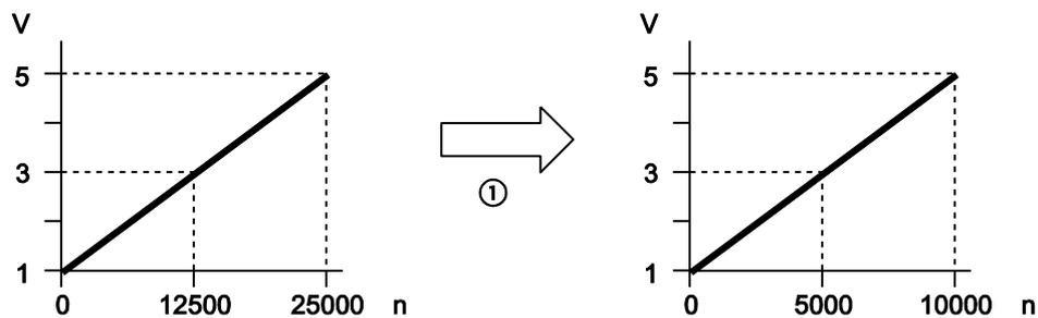
Scale conversion is executed on a channel-by-channel basis.
