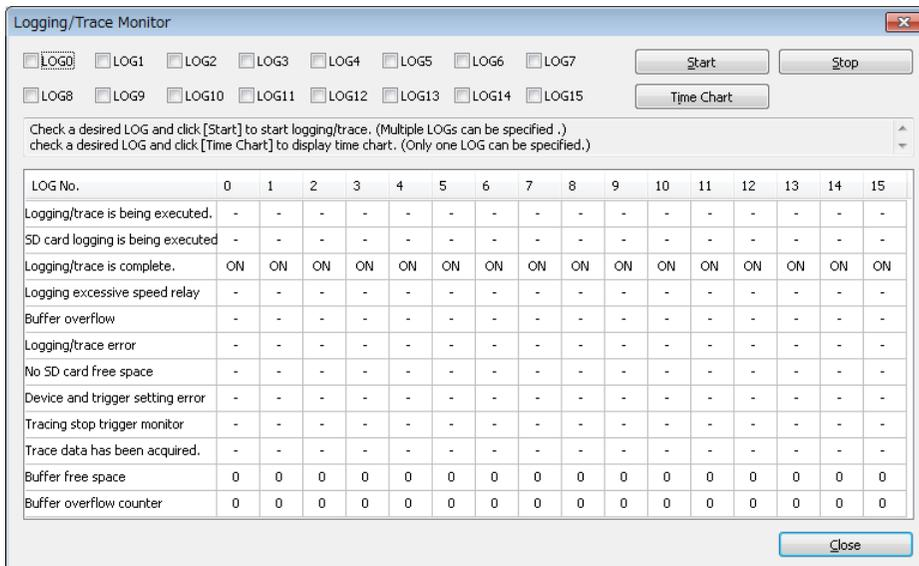
2. Check the box of a desired LOG number, and press the [Start] button.
