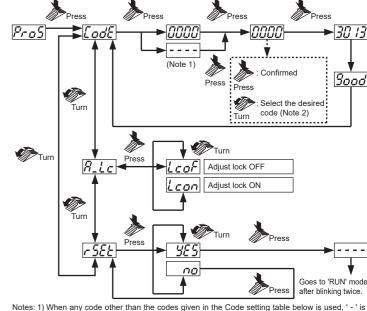
Notes: 1) When any code other than the codes given in the Code setting table below is used, ' - ' is displayed. The factory setting is 'ពូវជាម '. 2) When the code setting function is used, refer to the 'Code setting table' given below.
