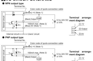
Internal circuit -Notes: 1) The guick-connection sub cable does not have +V (brown) and 0V (blue). The power is supplied from the connector of the main cable.
