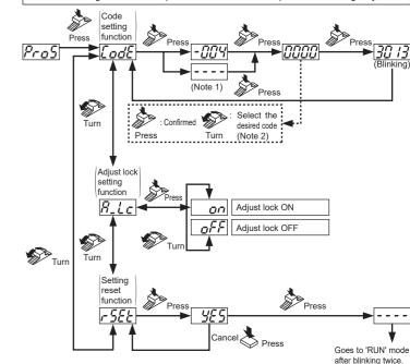
Notes: 1) When any code other than the codes given in the code setting table below is used, ' - ' is
