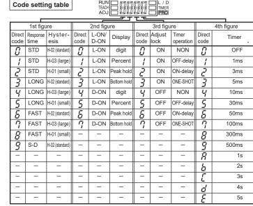
3) In order to change PRO mode setting to 'RUN' mode, press MODE key for 2 sec. or more. 4) The response time 'H-SP' cannot be set by using the code setting function
