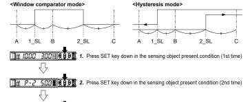
3. Press SET key down in the sensing object present condition (3rd time)
