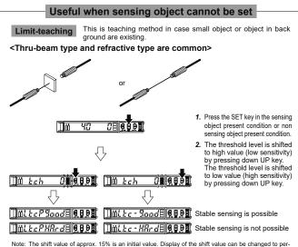
centage [approx. 0 to 999% (unit 1 %)] or incident light intensity [0 to 9999 (unit 1)]. For setting the shift amount, refer to <PRO1> in "PRO MODE OPERATION MANUAL."
