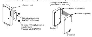
Notes: 1) HG-TSV10 is sold individually. Two HG-TSV10 units are required when installing to both emitter and receiver
