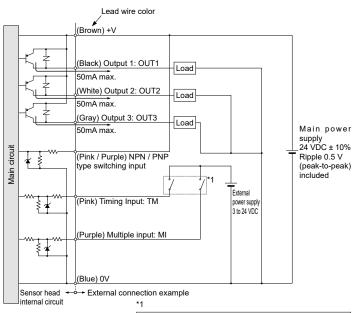
Non-voltage contact or PNP transistor open collector output IN o 0V o 0V < High [5V to 30V DC (inrush current of 0.04mA max.)]: Enabled Low [0 to 0.6V DC or open]: Disabled Refer to the HL-G1 Series User's
