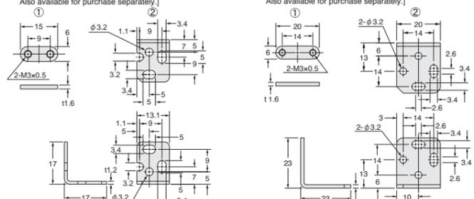
Material: Cold rolled carbon steel (SPCC) (Uni-chrome plated)
