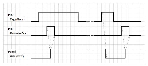
1. When an alarm condition is detected the HMI device set Ack Notify to 0 and all related actions are executed.
