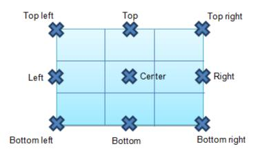
An algorithm finds a matching hot point among the near widgets hot points matching either the x or the y coordinates of the source snap point. For line widgets, the source snap points are the terminal points of the line.
