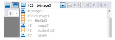
Important: Correct ordering of widgets is essential for runtime performance since overlapping dynamic widgets can invalidate static optimization and reduce performance of HMI applications.
