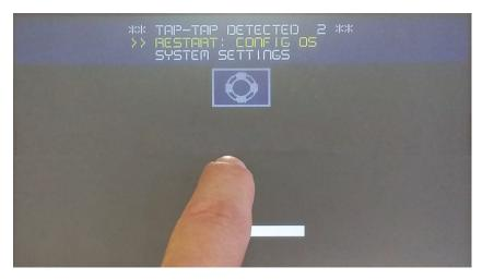
HMI will restart into System Settings in Config OS mode:
