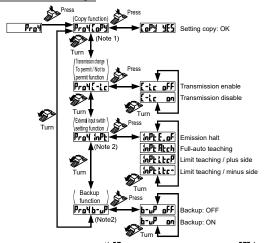
Notes:1) When the ultra high-speed ' N-5P' in the response time change function ' 5PEd' is set, the copy function can-
