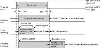
Notes:1) In the emission halt state, since the incident light intensity is judged as 0, the signal is output when the emission halt is confirmed (the trailing differential mode is selected) or the emission halt is canceled (the rising differential mode is selected) in the differential mode.
