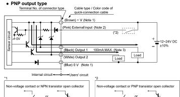
Notes :1)The quick-connection sub cable does not have +V (brown) and 0V (blue).The power is supplied from the connector of the main cable.
