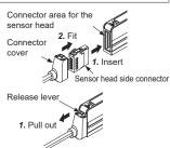
Note: Do not pull by holding the cable without pressing the release lever, as this can cause cable break or connector break.
