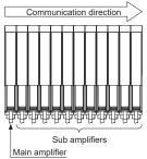
When this product and other products (e.g. fiber sensor amplifiers, pressure sensor controllers, etc.) are connected together in cascade, install those products so that they are in order of Group A, B, D and C as shown in the right figure. This product is included in Group D.
