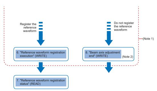
Notes: 1) The inside of the frame indicated by the red dotted lines represents beam axis adjustment mode.
