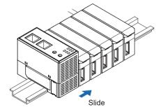
4. Attach end plates **MS-DIN-E** (optional) with the flat side facing in so as to enclose the connected units at the ends.
