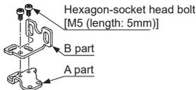
1. Fix the standard mounting bracket with two hexagon-socket head bolts [M3 (length: 5mm)]. The tightening torque should be 0.6N·m or less.
