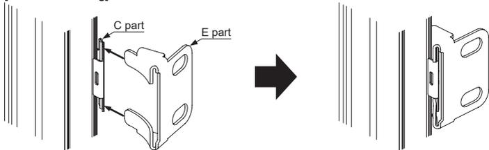
3. Mount the D part or E part on to the mounting surface with the two hexagon-socket head bolts [M5 (purchase separately)].
