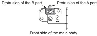
4. Mount the mounting bracket on to the mounting surface with two hexagon-socket head bolts [M5 (purchase separately)] temporarily.
