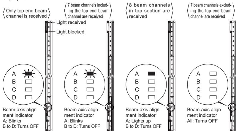
When all the 8 beam channels divided into each section are received, the beam-axis alignment indicator lights up in red. The indicators corresponding to the different sections light up in red, one by one, when the beam channels of the respective sections are received. When all the beam channels are received and the control output (OSSD 1 / 2) turns ON, all the four indicators of the beam-axis alignment indicator turn into green.
