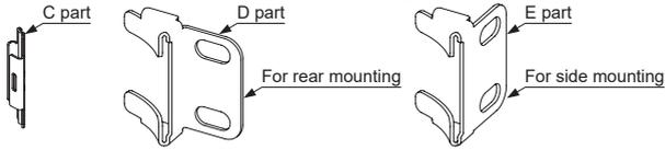
1. Hook the C part into the groove on the side of the body and press it.
