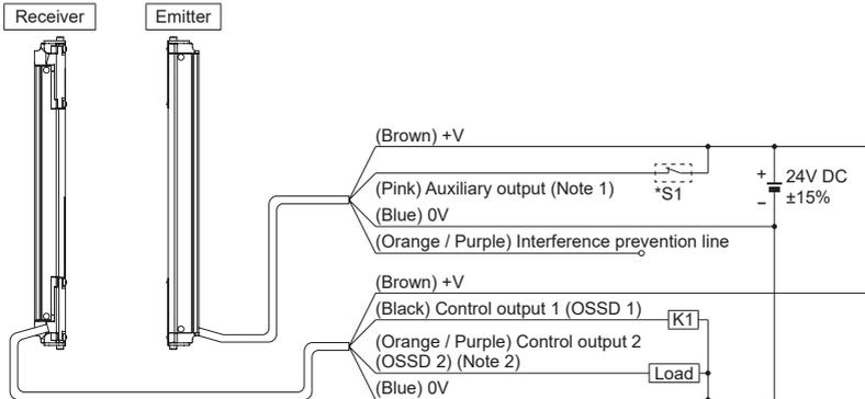
Notes: 1) The figure above shows the connection pattern for the SF1-CC□A. The pink cable is not used for the NA40-CC□.
