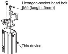
2. For side mounting, remove the B part.
