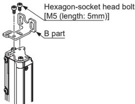
3. Mount the brackets so that the protrusion of the A part and the B part are overlapped. B part to be attached to the top or bottom side of this device differs depending on the direction of mounting described as the following chart.
