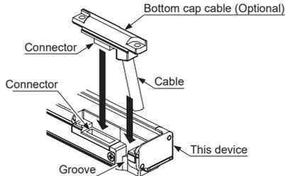
2. Tighten the two M3 screws. The tightening torque should be 0.3N·m or less.
