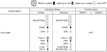
Note: The status of the emitter / receiver indicators during operation above shows the case in PNP output setting mode. In case of NPN output setting mode, the NPN indicator (orange) lights up.
