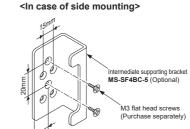
2. Insert this device into the intermediate supporting bracket.
