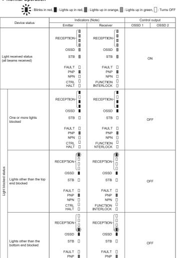
Note: The status of the emitter / receiver indicators during operation above shows the case in PNP output setting mode. In case of NPN output setting mode, the NPN indicator (orange) lights up.
