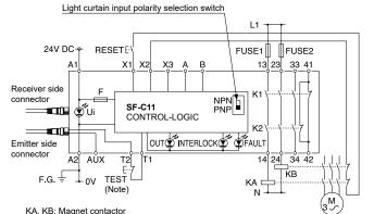
Note: Emission halt occurs when the test (TEST) button is open, and emission occurs when the test (TEST) button is short-circuited. If not using the test (TEST) button, short-
