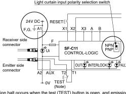
Note: Emission halt occurs when the test (TEST) button is open, and emission occurs when the test (TEST) button is short-circuited. If not using the test (TEST) button, short-
