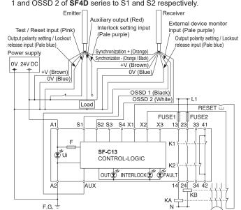
• In case of connecting Type 2 PNP output type SF2C series, connect the control output (OSSD) of SF2C series to S1, and also put a jumper
