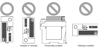
In addition, make sure that the device's upper lower, left, and right surfaces are spaced by a 50mm or more from surrounding objects such as other devices and wiring ducts
