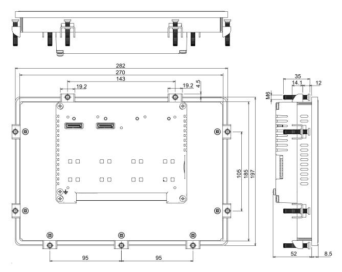
Unit: mm Tolerance (except T): ±1 T Tolerance: ±0.5
