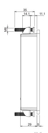
Unit: mm Tolerance (except T): ±1 T Tolerance: ±0.5
