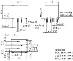
\* Dimensions (thickness and width) of terminal is measured after pre-soldering. Intervals between terminals is measured at A surface level.
