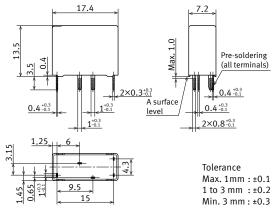
\* Dimensions (thickness and width) of is measured after pre-soldering.
