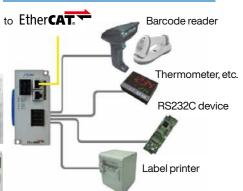
\* IO-Link, Modbus, Serially controlled devices such as RS-232C and RS-485 devices are converted to EtherCAT. EtherCAT can be installed without putting old assets to waste.
