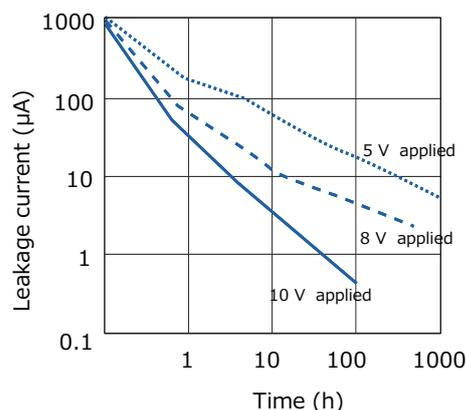
※ To make the recovery of LC values easy to show, samples that LC values have been increased on purpose are used in the test.
