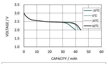
Charging Condition :  $CV(3.1V,160\Omega,60H)$ Discharging Condition :  $CR(20k\Omega, 2.0V \text{ Cut-off})$
