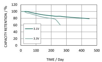
Charging Condition : CV(3.1V or 3.3V,60°C) Discharging Condition : CR(1.5k $\Omega$ , 2.0V Cut-off, 60°C)
