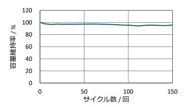
Charging Condition: CV(2.3V, 750Ω, 8H, 20°C) Discharging Condition : CR(10k $\Omega$ , 1.0V Cut-off, 20°C)
