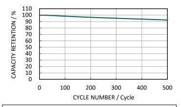
Charge Condition: CC/CV 30.0mA(1.0C) - 4.35V, 1.5mA(0.05C) cut-off at  $20^{\circ}$ C Discharge Condition: CC, 30.0mA(1.0C) - 3.0V cut-off at  $20^{\circ}$ C
