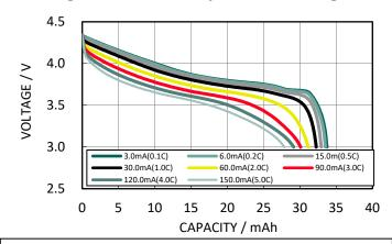
Charge Condition: CC/CV 30.0mA(1.0C) - 4.35V, 1.5mA(0.05C) cut-off at  $20^{\circ}$ C Discharge Condition: CC, 3.0V cut-off at  $20^{\circ}$ C
