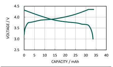
Charge Condition: CC/CV 30.0mA(1.0C) - 4.35V, 1.5mA(0.05C) cut-off at  $20^{\circ}$ C Discharge Condition: CC, 6.0mA(0.2C) - 3.0V cut-off at  $20^{\circ}$ C
